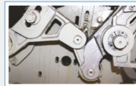
The 6 Connecting Rod Weft Insertion Mechanism
